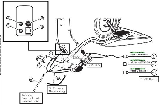
Note to the TV Installer: This reminder is provided to call the TV system installer's attention to Article 820-40 of the National Electric Code that provides guidelines for proper grounding and, in particular, specifies that the cable ground shall be connected to the grounding system of the building as close to the point of cable entry as practical.
